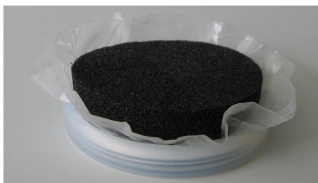
Changing the Membrane - Inserting
